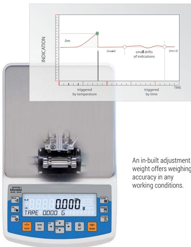
An in-built adjustment weight offers weighing accuracy in any working conditions.
