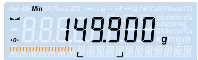
Mass value lower than the value of minimum threshold
